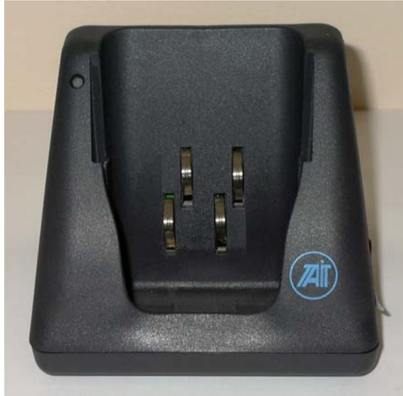
Turn the charger over. The serial number, product code and software version is on the bottom side of charger unit.
