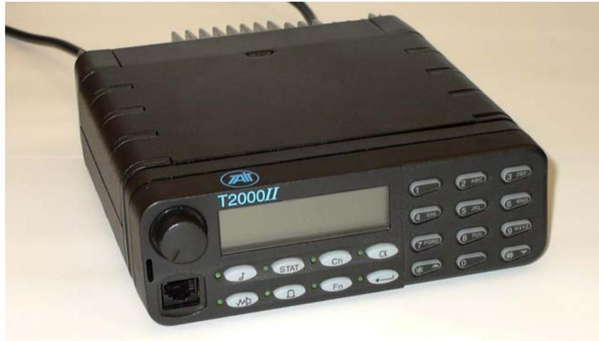
The serial number and product code are located on the radio's heatsink at the rear left of the radio (looking from front on).
